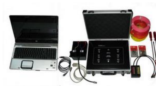
Figure 1. S-Field automatic multichannel resistivity tool
